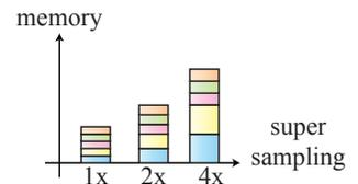
**Figure 4:** While the G-buffer stores all shading data at full supersampled resolution, we introduce a visibility buffer which references compact shading data buffers. Due to shading reuse the size of the compact buffers does not scale with the supersampling density.
