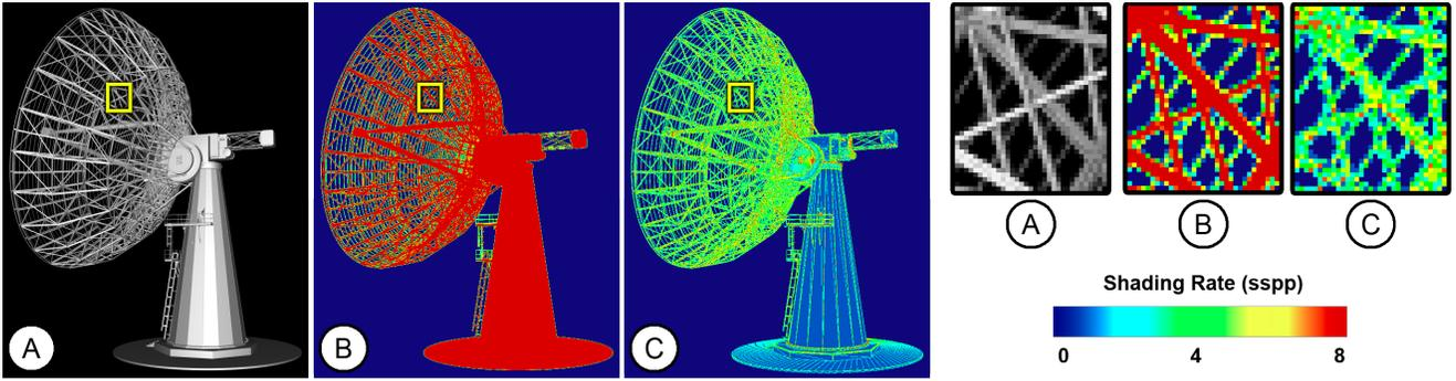
**Figure 6:** In order to achieve the same antialiasing quality as with  $8\times$  MSAA (A), standard deferred shading needs to evaluate shading at  $8\times$  supersampling (B). Our method stores and evaluates shading at significantly lower rates (C), but keeps the antialiasing quality by supersampling visibility. The heat maps visualize the number of shading samples per pixel.
