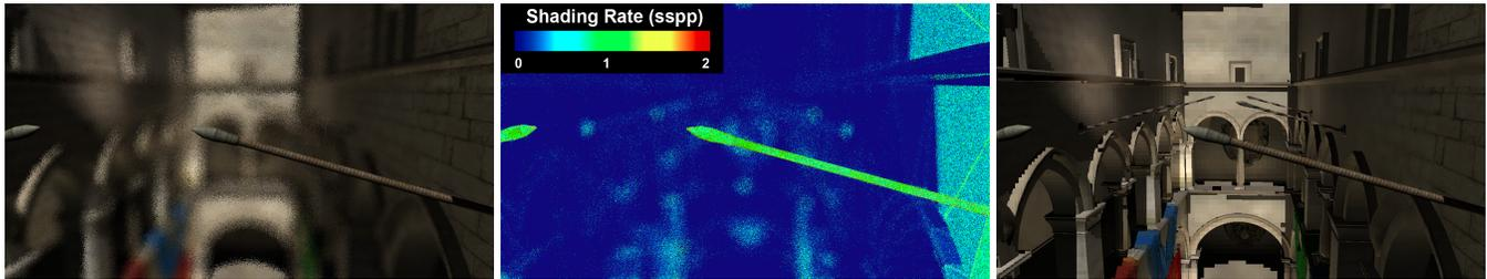
**Figure 1:** Decoupled deferred shading enables efficient shading reuse for stochastic rasterization. These images show depth of field rendering with  $4\times$  visibility supersampling (left), a visualization of the shading rate (sspp—shading samples per pixel, center), and the same shading as seen from a pin-hole camera (right). Our adaptive scheme reduces the shading frequency of defocused regions.
