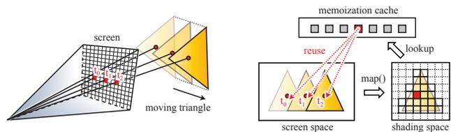
**Figure 2:** (a) A moving surface point is visible at multiple locations over time on the screen. Assuming the time  $t_2 - t_0$  is small enough, the same shaded color can be used for all screen samples. (b) Decoupled sampling samples visibility and shading in different domains. The method reuses recent shading samples from a memoization cache, mapping multiple visibility samples to a single sample in shading space.
