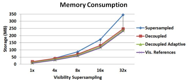
**Figure 9:** Storage requirements of the CG-buffer compared to standard G-buffers. Our memory footprint consists of visibility and shading samples. The lightweight visibility data saves significant space at high supersampling resolutions, and note that the footprint of shading samples becomes negligible (we also plotted the space used for storing visibility references only). The Sponza scene was rendered at  $1280\times 720$  pixels.
