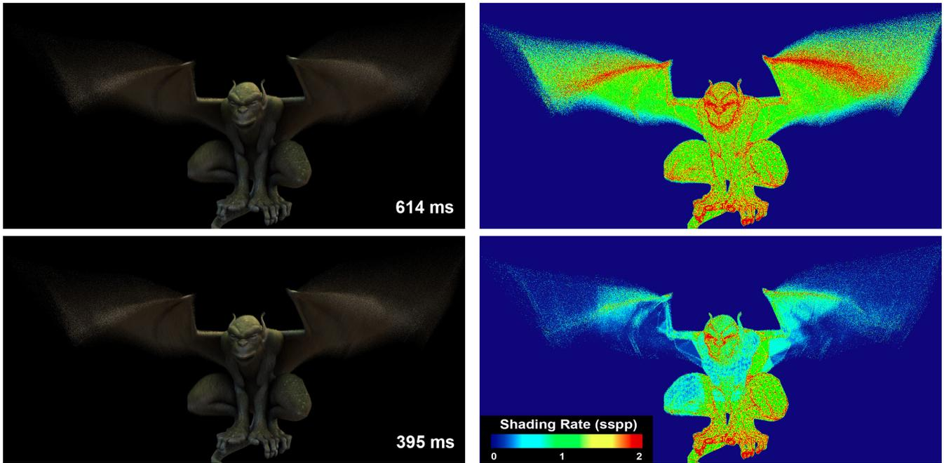
**Figure 7:** A motion blurred character rasterized with  $8\times$  stochastic supersampling. Deferred shading is computed using 36 ambient occlusion rays per shading sample (using OptiX). Due to decoupled sampling, the shading rate stays close to 1 sspp despite the high sample count (top row). Adaptive shading (bottom row) saves  $\sim 30\%$  of the rendering time by further decreasing the shading rate of fast-moving surfaces.
