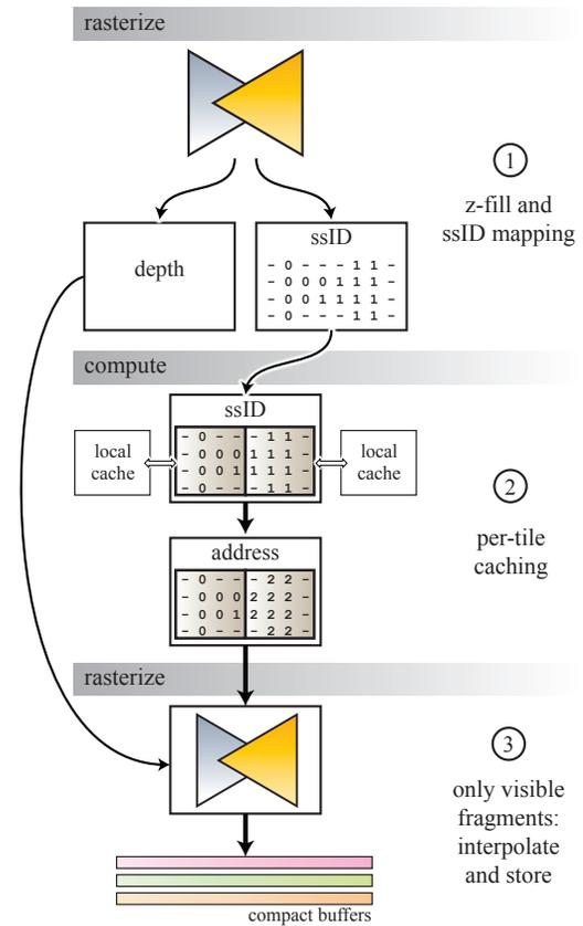
**Figure 5:** The outline of the multi-pass decoupled shading algorithm. Note, that for simplicity we use assume flat-shaded triangles (no interpolation). The example also shows that shading samples visible at multiple tiles are redundantly stored. The major benefit of this method is the speed of the local cache.
