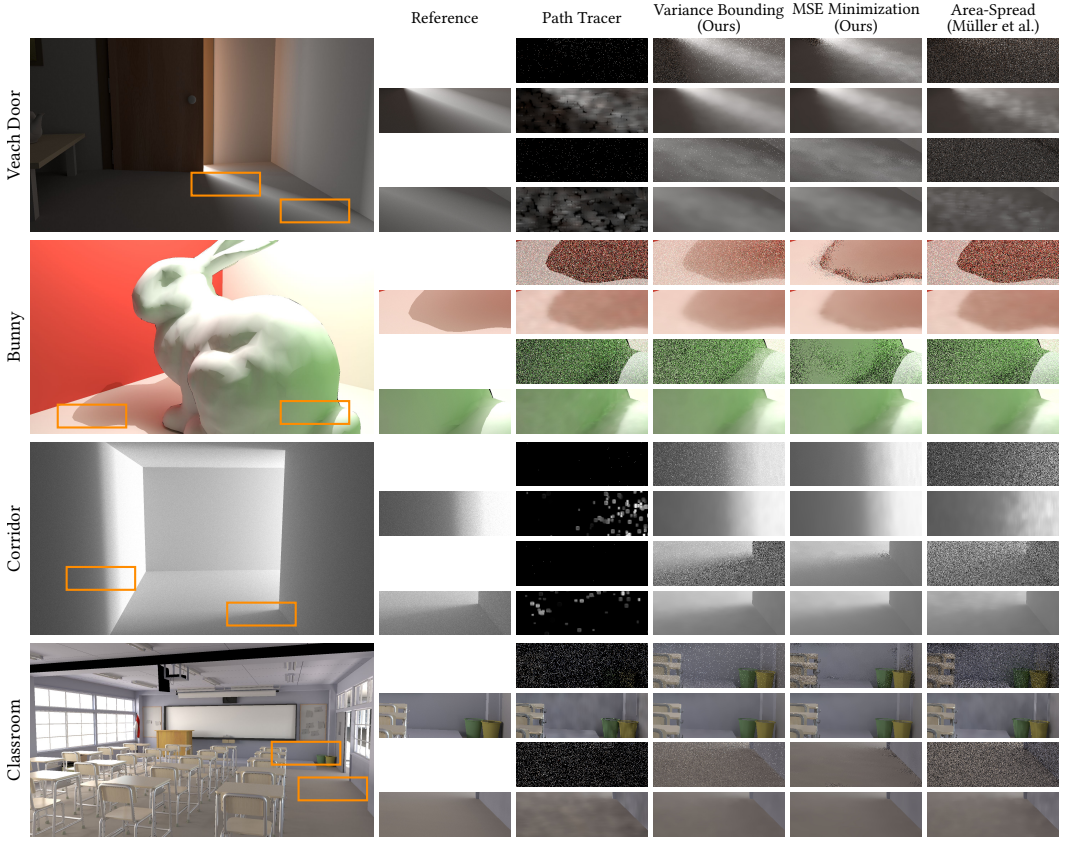
Fig. 10. Equal-sample comparison of termination strategies with and without denoising for different scenes: The plain path tracer vs. our variance bounding (relative variance threshold t = 1.0 ) vs. our MSE minimization (sample target s = 100 ) vs. the area-spread heuristic ( c = 0.01 ). The first row shows the 1spp output, the second row the output of the denoiser [Schied et al. 2017] after four still frames.
