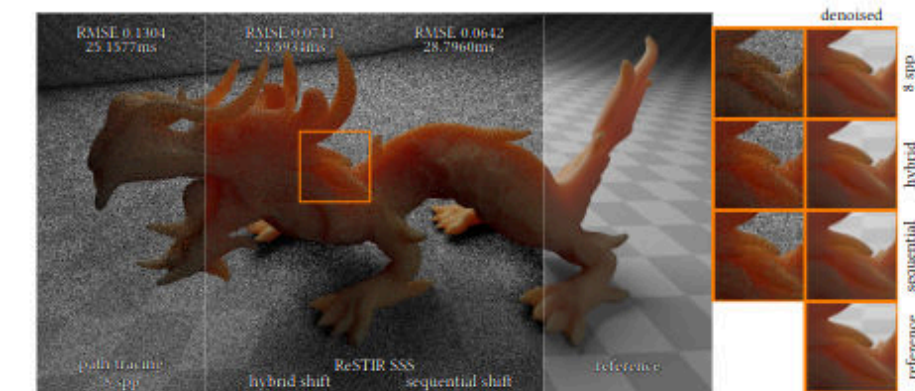
Fig. 1. A dragon with a material that exhibits noticeable subsurface scattering. We apply ReSTIR for subsurface scattering using our hybrid and sequential shift in real-time path tracing to significantly reduce noise and denoising artifacts in regions with visible scattered light.
