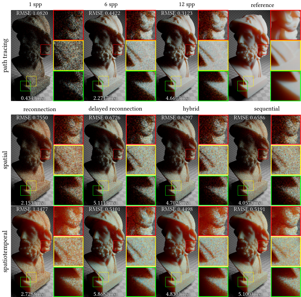
Fig. 4. Scene with a highly scattering object and a single large light source. Comparison between standard path tracing and ReSTIR SSS with spatial and spatiotemporal reuse.
