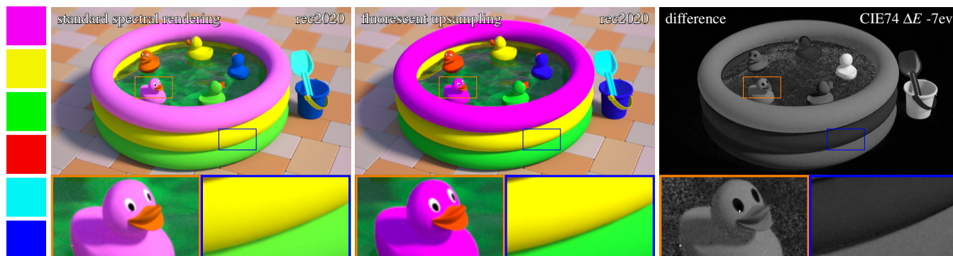
Figure 1: A spectrally rendered scene with standard RGB to spectrum upsampling (left) cannot achieve reflectance spectra with arbitrary colour saturation and brightness due to energy conservation constraints. Our technique (centre) converts bright and deeply saturated input RGB colours to regular reflectance spectra and enhances them with a fluorescent component, reproducing colours from a considerably wider gamut. The input colours were specified in ACEScG—for instance, the top ring of the swimming pool has color (0.9, 0, 0.9) in ACEScG. To visualise colours of such high saturation, we interpret the rec2020 data of the rendered images as sRGB for display, and we also provide a display-independent difference image in CIE74 \Delta E on the right (stopped down by 7ev, i.e. a saturated pixel value of 1.0 corresponds to \Delta E = 128 ). Similarly, the squares to the left visualise the ACEScG input colours reinterpreted as sRGB.
