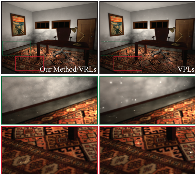
Figure 11: These images show volume-to-surface transport in the SMOKY ROOM scene computed in only 600s; some regions are dark also due to absorption and out-scattering in the participating media. The close-ups compare the singularities of VRLs and VPLs (both without clamping).
